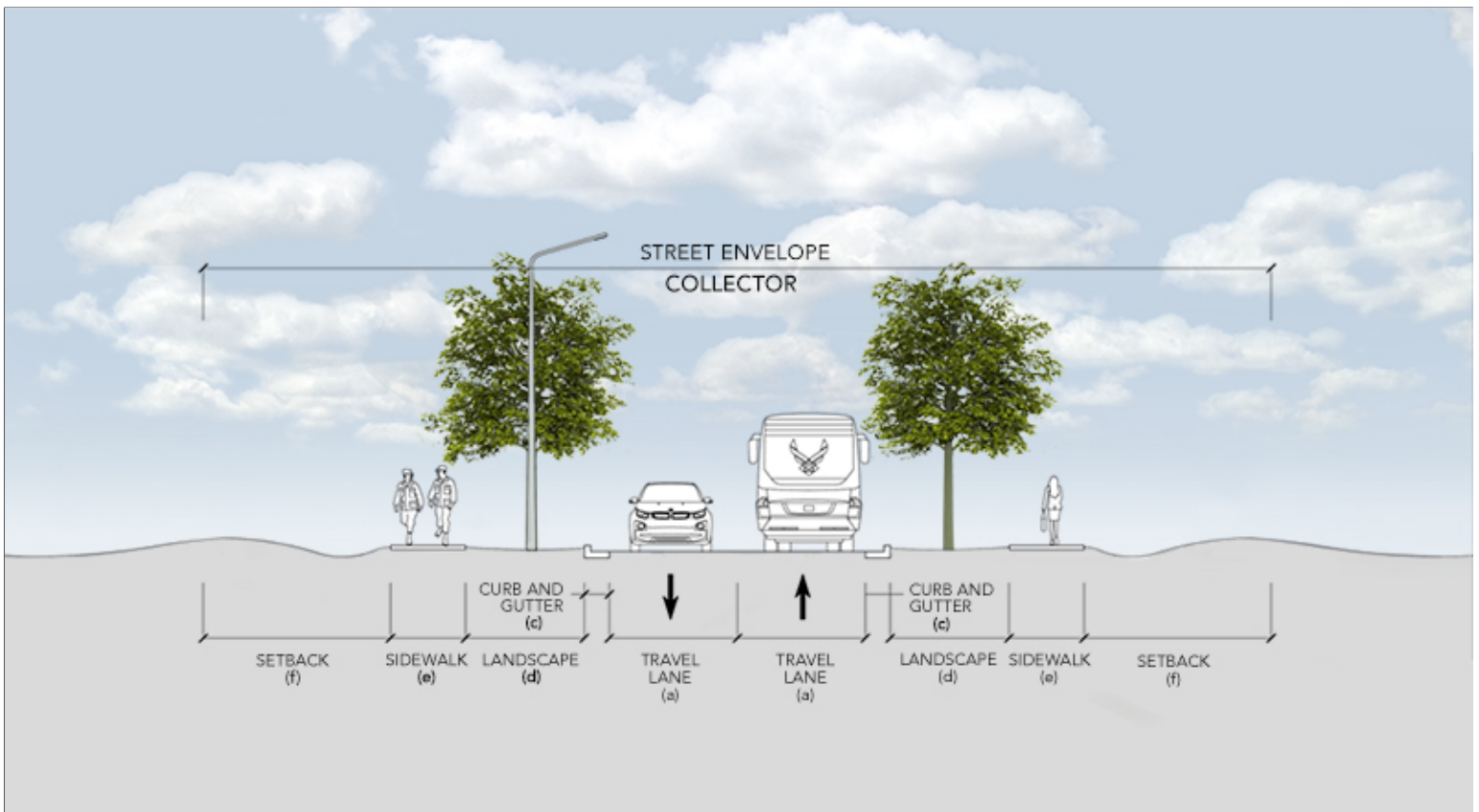
Travel Lane (a): 12' Median (b): N/A Curb and Gutter (c): 2' Landscape (d): 10' Sidewalk (e): 6' Setback (f): 15' or per AFTP requirements
