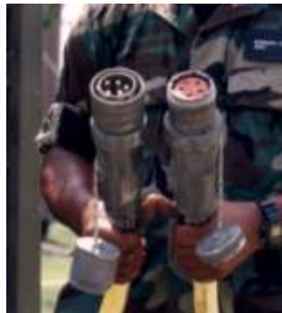
Figure 2.15. Low-Voltage Cables with Cannon Plug Connections.
