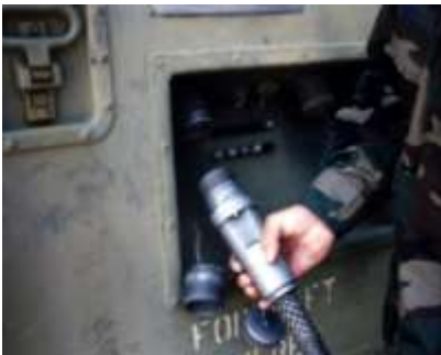
Figure 4.18. Cannon Plug Connection from SDC to ESC Service Panel.
