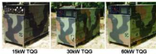
Figure 2.6. Tactical Quiet Generators.
