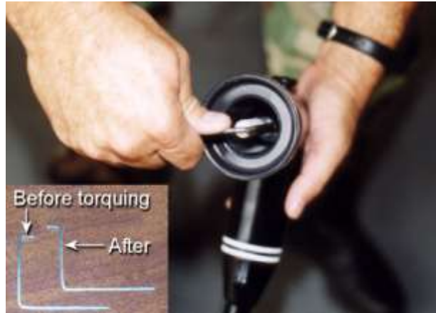
Figure A2.18. Wrap the End of the Elbow for Protection.
