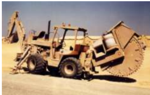
Figure 4.7. Tractor with Backhoe, Blade, and Trenching Wheel.
