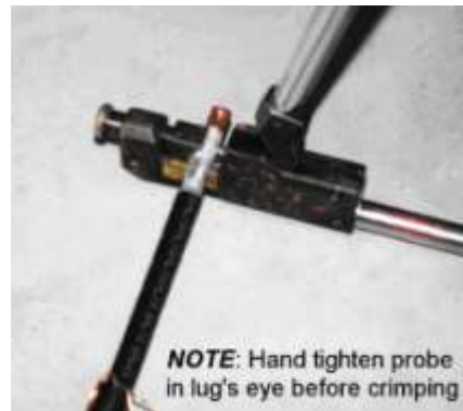
Figure A2.13. Crimping Compression Lug.
