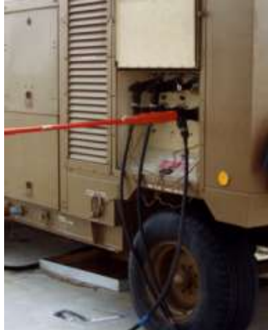
Figure 5.19. Connecting Cables to MEP-12A with Grip-All Clamp Stick.
