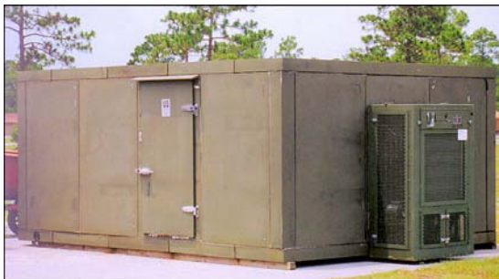
Figure 5.9. 1200-CF Refrigeration Unit.
