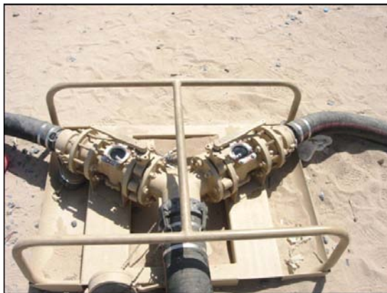
Figure 7.5. Tactical Automated Service Station (TASS).
