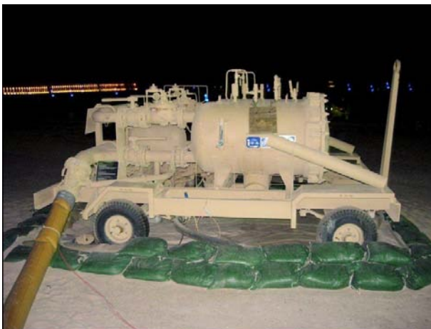
Figure 7.2. R-19 Trailer-Mounted Filter Separator.
