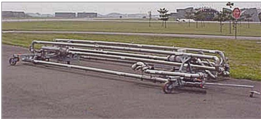
Figure 7.9. GRU-17E Aircraft Fuel-Servicing Unit.
