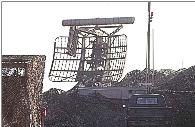
Figure 7.14. Landing Control Central Surveillance Radar System.
