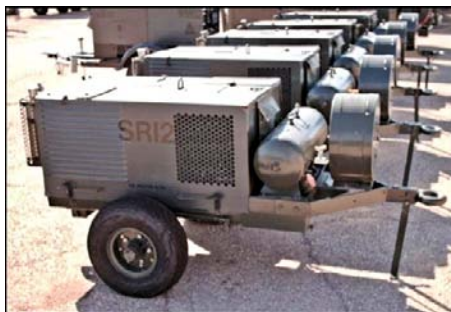
Figure 6.5. MC-2A Diesel-Driven Air Compressor.
