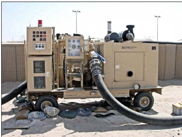
Figure 7.2. R-19 Trailer-Mounted Filter Separator.
