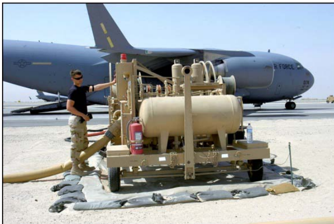
Figure 7.3. R-20 Multi-Aircraft Servicing Platform.
