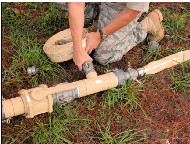
Figure 3.14. Water System Hoses, Connectors and Valves.
