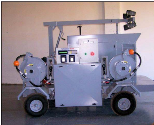
Figure 7.5. Tactical Automated Service Station (TASS).
