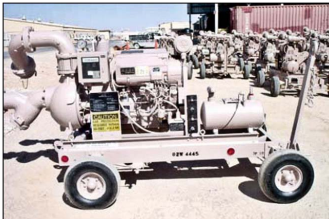
Figure 7.7. R-22 Trailer-Mounted Transfer Pump.
