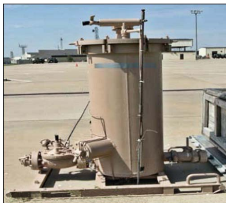
Figure 7.8. FFU-15E Skid-Mounted Filter Separator.
