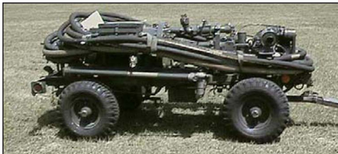
Figure 7.10. PMU-27M Pumping Assembly.
