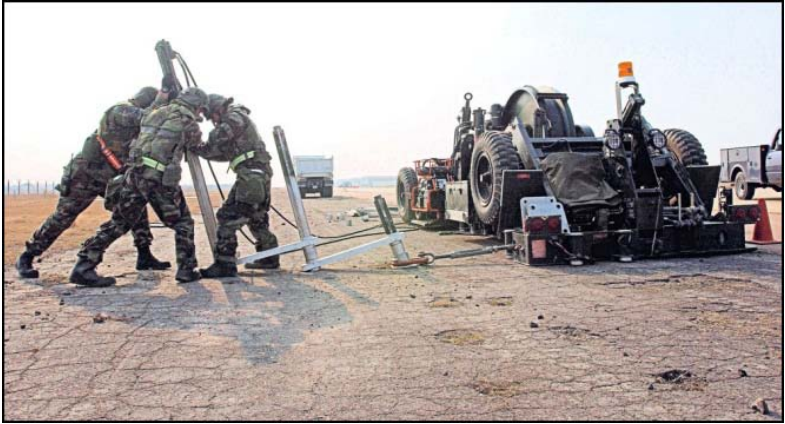
Figure 6.7. Mobile Aircraft Arresting System.
