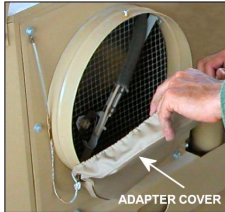
Figure 5.13. Adapter Cover Installation.
