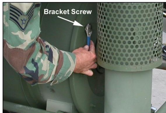
Figure 2.18. Smoke Stack Bracket Screw.
