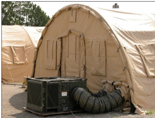
Figure 4.1. Field Deployable Environmental Control Unit (FDECU).
