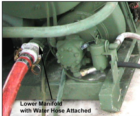
Figure 2.12. Lower Manifold Assembly.
