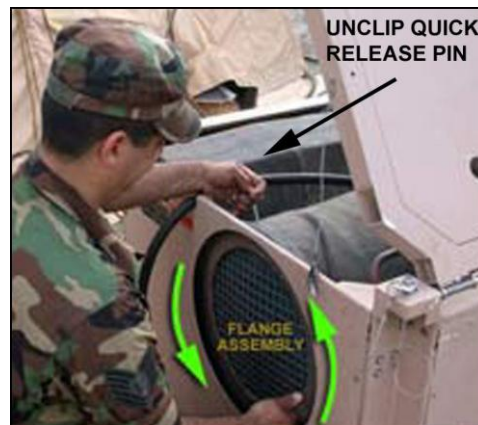
Figure 4.12. Return Air Flange Assembly Removal.
