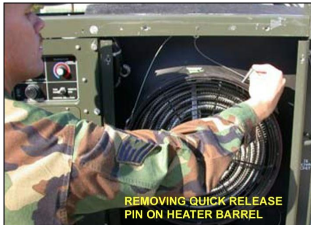
Figure 4.15. Removal of Quick Release Pins on Heater Barrel.
