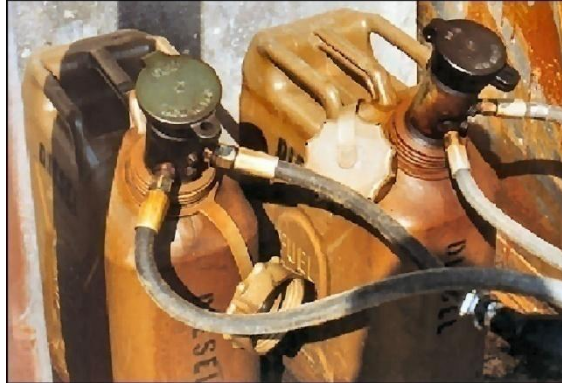
Figure 2.3. Drum Fill Adapter and Flexible Hoses on Fuel Cans.
