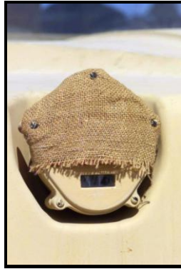
Figure 7.2. Burlap Covering Headlight.
