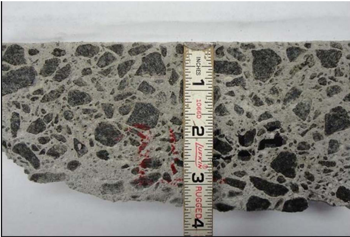
Figure 27. Example from Test Slot of Acceptable Aggregate Distribution, No Segregation and Minimal Surface Paste with Traprock
