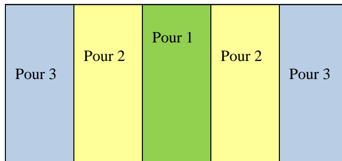
Figure 9. Mandatory HTC Placing Sequence
