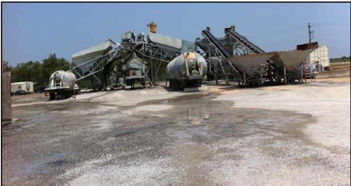
Figure 5. Duke Field On-Site Batch Plant (Horizontal Shaft Type)
