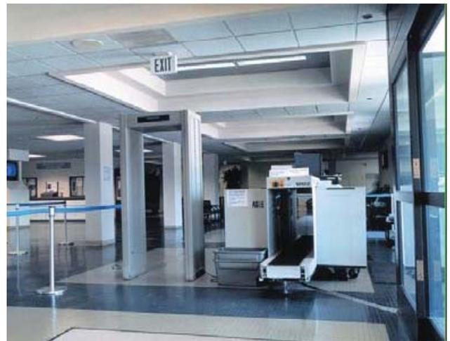
*X-Ray and Magnetometer Equipment for Security Screening*
