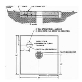
Figure D-1 Valve Box with Disk
