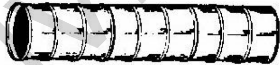
Barrel No. 3 Length = 105 inches Opening = 23 inches
