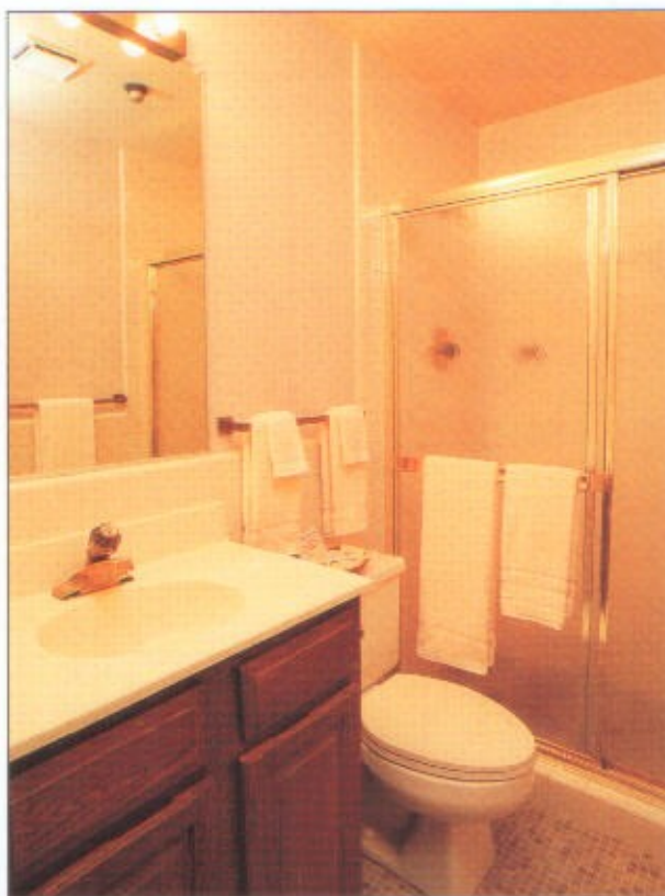
Use ceramic tile flooring and wainscotting or heavy sheet vinyl on bathroom floor.
