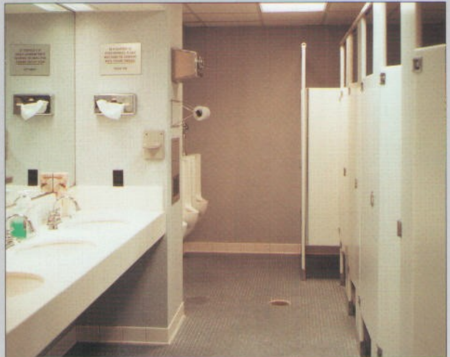
Install tile floors for restrooms and durable type II vinyl wallcovering or tile for walls.
