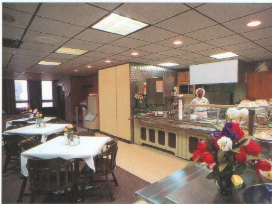
The serving line should include tray and silverware storage bins, an entree serving line with steam heat or ice trays, and sneeze guards or other protective surfaces.
