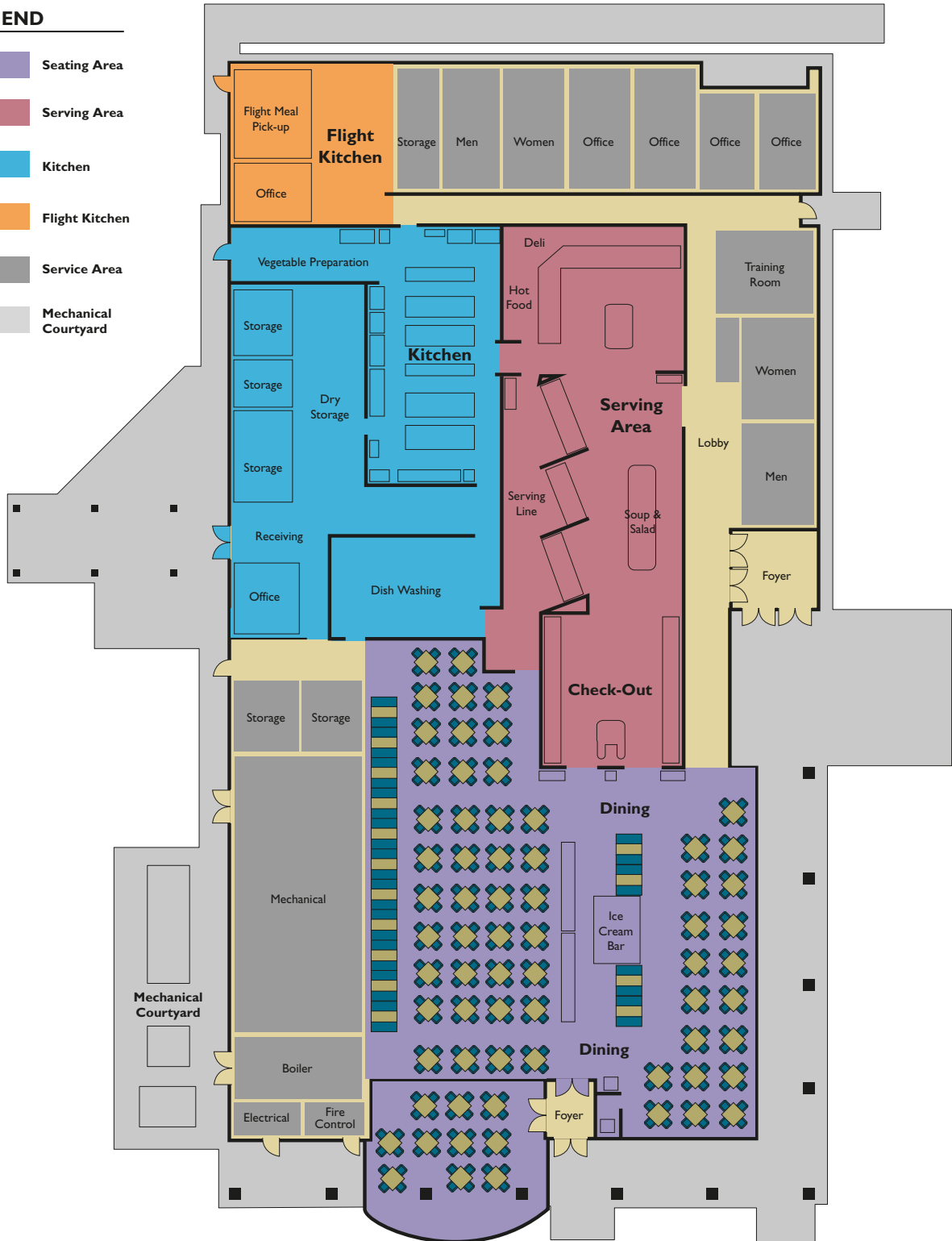
New Dining Facility Floorplan at Eglin AFB
