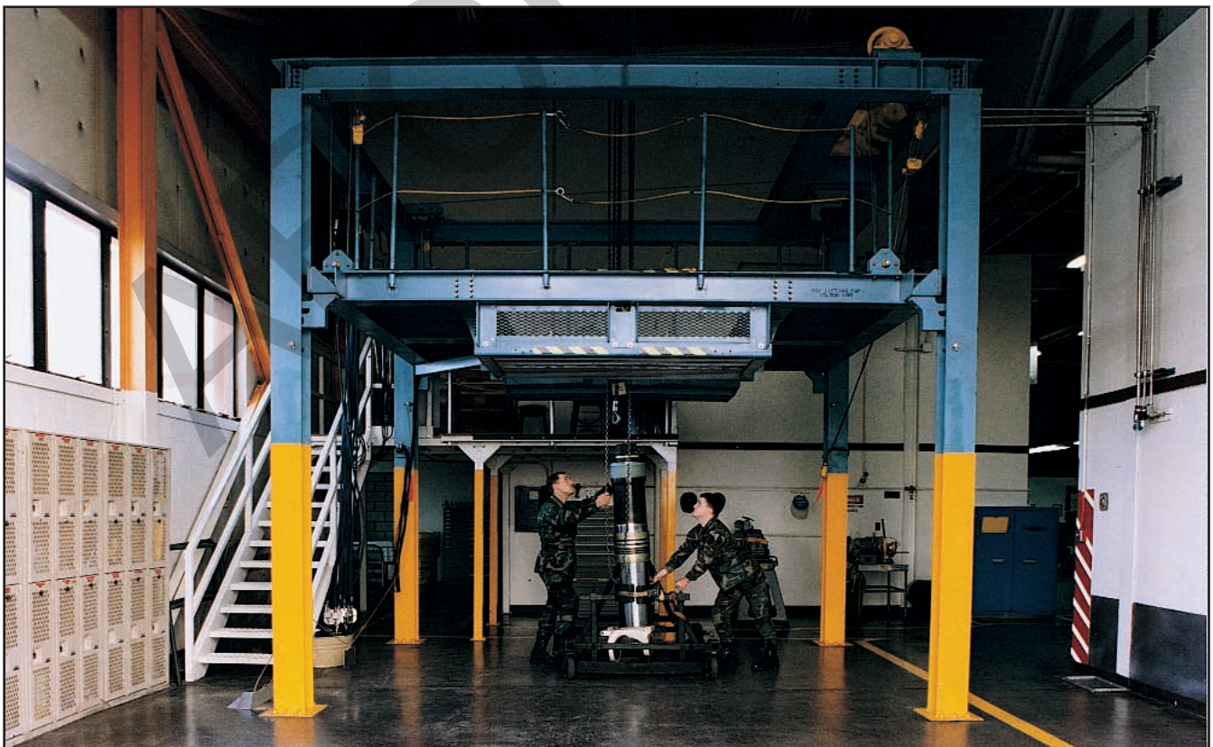
The C-5 landing gear test stand requires a high bay for maintenance and testing activities.
