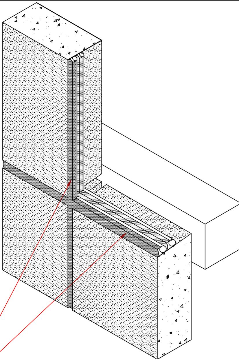
INSTALL 2-STAGE VERTICAL AND HORIZONTAL SEALANT JOINTS WITH THE APPROPRIATE SIZED BACKER ROD. TWISTED BACKER ROD IS NOT TO BE USED. PRIME ALL SUBSTRATES WITH THE APPROPRIATE MANUFACTURER'S PRIMER. ALLOW THE BACK JOINT TO CURE BEFORE INSTALLING THE SECOND STAGE WEATHER SEAL JOINT. THE VERTICAL SECOND STAGE JOINT IS TO BE RETURNED TO THE VERTICAL FIRST STAGE JOINT AND WEEPED PER INDUSTRY STANDARDS.
