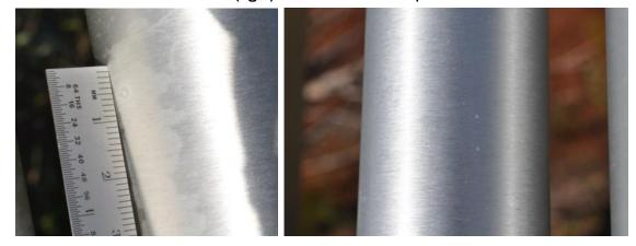
Figure 33. FRP railing coupon at FRF (left) and KTA (right) after 12 months of exposure.
