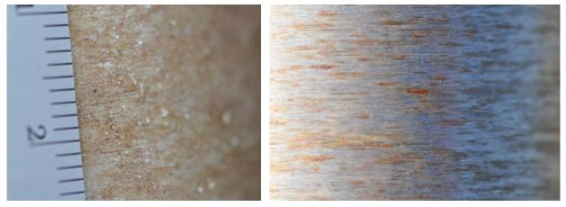
Figure 35. Stainless steel railing coupon at FRF (left) and KTA (right) after 12 months of exposure.
