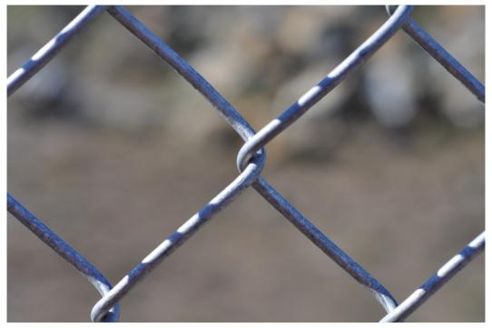
Figure A11. Aluminized after 6 months exposure.
