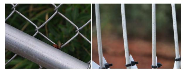
Figure B74. (Left) Alumiunm fabricated fencing. (Right) Aluminum Wire Coupons
