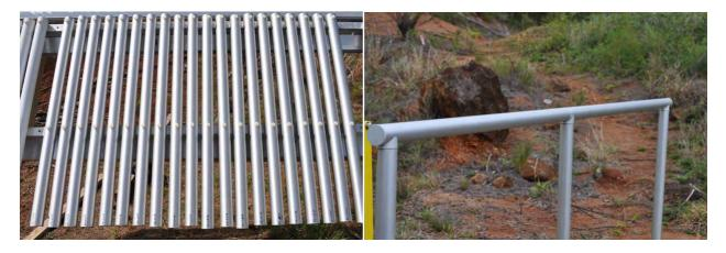
*Figure B69.* (Left) Aluminum railing coupons. (Right) Aluminum railing test section.
