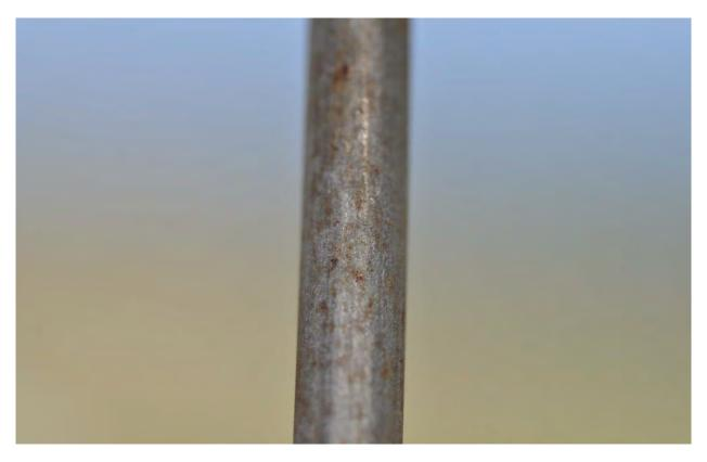
Figure B114. Stainless Steel Wire Coupon
