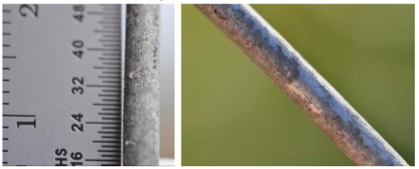
Figure 25. Fuse bonded PVC coated wire coupon at FRF (left) and KTA (right) after 12 months of exposure.
