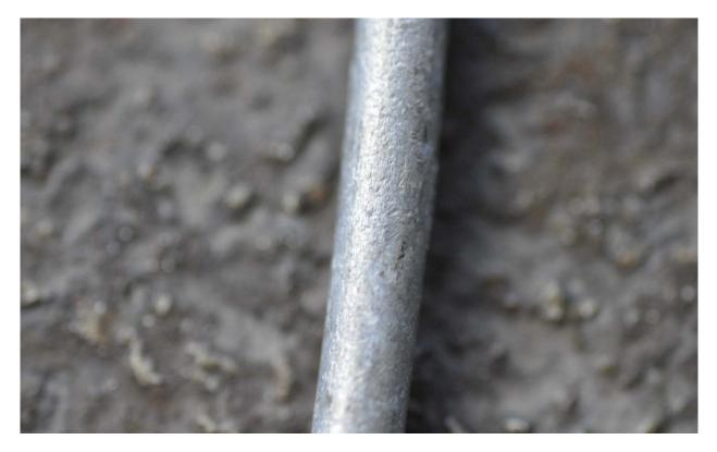
Figure B128. Aluminized Steel Wire Coupon
