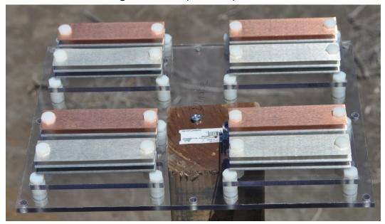
Figure A5. Atmospheric coupon rack.
