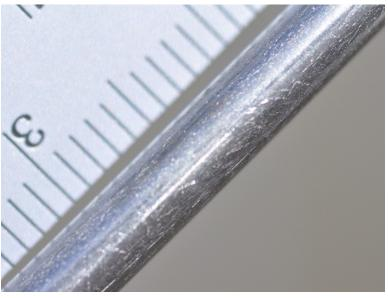
Figure A18. Aluminum 6061 T6 after 12 months exposure.
