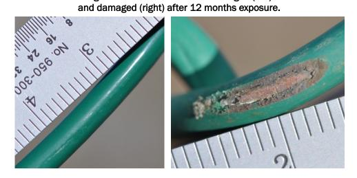
Figure A15. Standard PVC undamaged (left)
