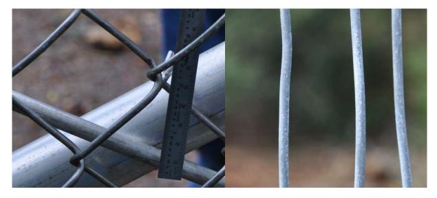
Figure B73. (Left) Galfan fabricated fencing. (Right) Galfan Wire Coupons
