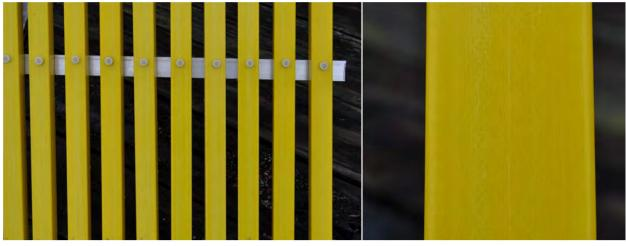
Figure B149. FRP Railing Coupon
