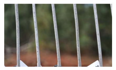
Figure B75. Standard galvanized wire coupons
