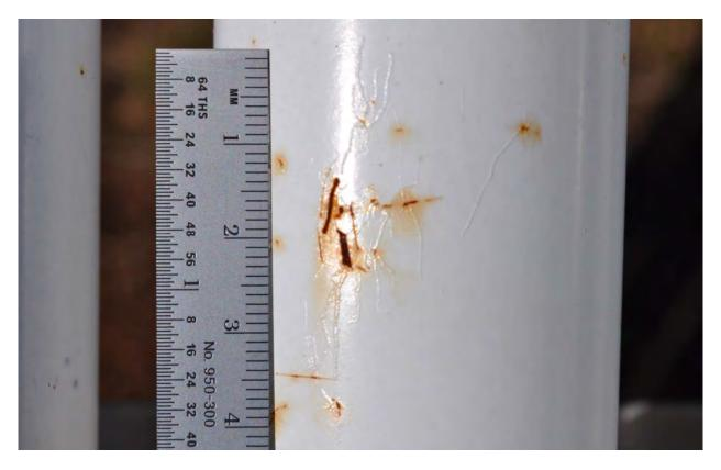
Figure B79. Coated Steel Coupon
