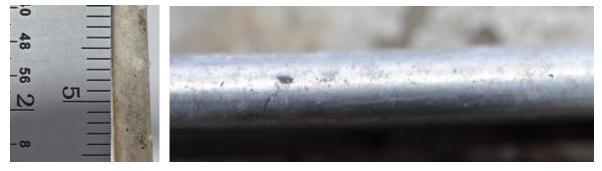
Figure 27. Stainless Steel wire coupon at FRF (left) and KTA (right) after 12 months of exposure.
