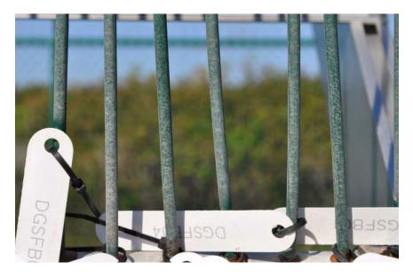
Figure B34. Fuse Bonded PVC Coated Galvanized Wire Coupon
