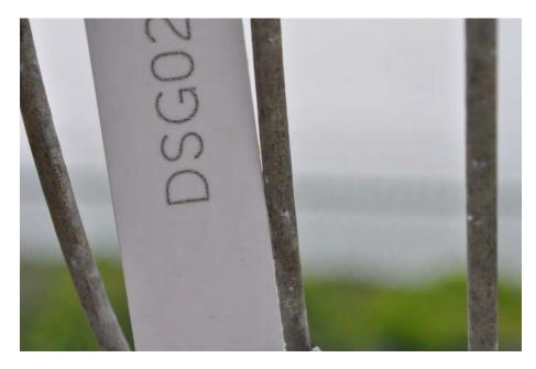
Figure B11. Standard Galvanized Wire Coupon
