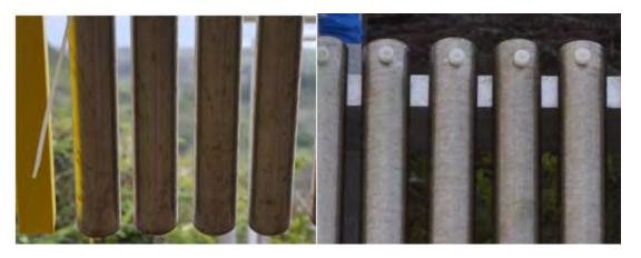
*Figure B66.* (Left) Stainless steel coupons facing away from the ocean; (Right) stainless steel coupons facing the Ocean.
