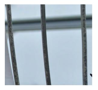
Figure B13. Aluminized Steel Wire Coupon
