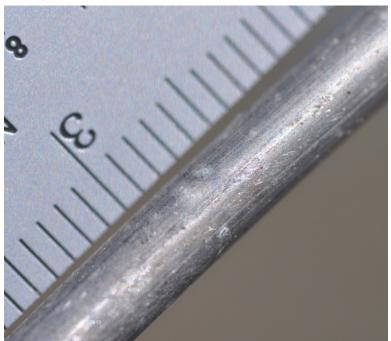
Figure A20. Stainless steel after 12 months exposure.
