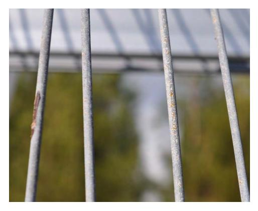
Figure B86. Standard Galvanized Wire Coupon
