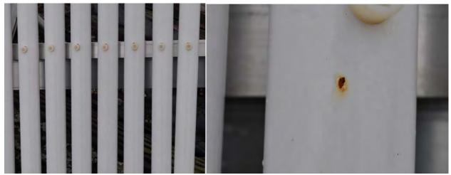
Figure B150. Coated Steel Coupon
