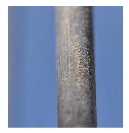
Figure B106. Standard Galvanized Wire Coupon
