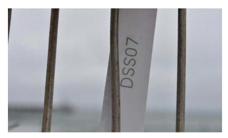
Figure B19. Stainless Steel Wire Coupon
