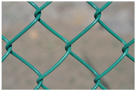
Figure A7. Fuse-bonded PVC after 6 months exposure.
