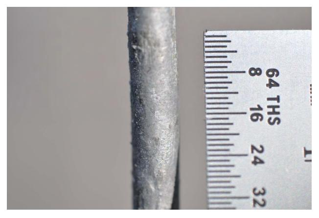
Figure B166. Aluminized Steel Wire Coupon
