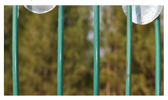
Figure B90. Fuse Bonded PVC Coated Galvanized Wire Coupon
