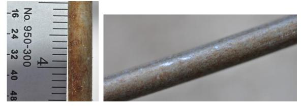
Figure 28. Galfan wire coupon at FRF (left) and KTA (right) after 12 months of exposure.
