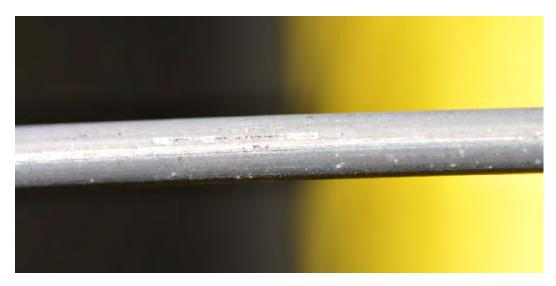
Figure B176. Standard Galvanized Wire Coupon
