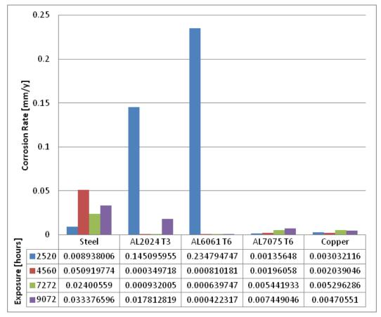
Figure A21. Corrosion rates of steel, copper and aluminum alloy atmospheric coupons after 3, 6, 9 and 12 months of exposure at PTA.
