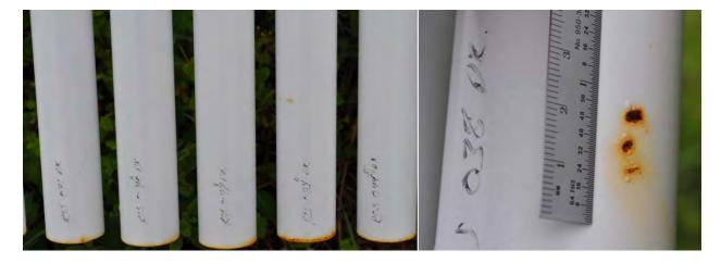
Figure B3. Coated Steel Coupon
