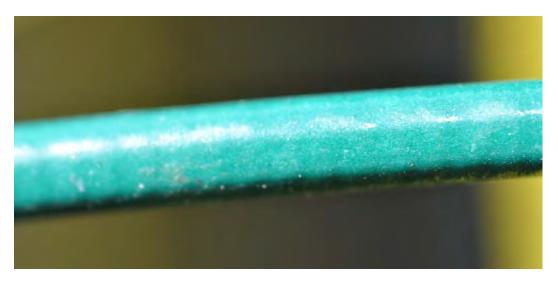
Figure B178. Fuse Bonded PVC Coated Galvanized Wire Coupon
