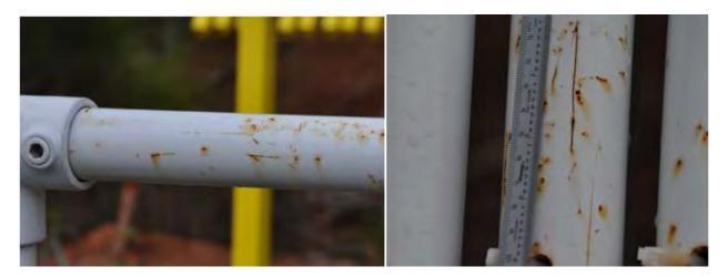
*Figure B67.* (Left) Painted carbon steel railing coating failure. (Right) Painted carbon steal coupon coating failure.
