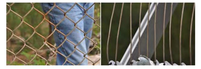
*Figure B70.* (Left) Stainless steel fence after 3 months exposure. (Right)Stainless steel wire coupons after 3 months exposure.
