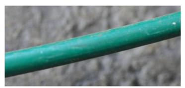
Figure 26. Aluminum wire coupon at the FRF (left) and KTA (right) after 12 months of exposure.
