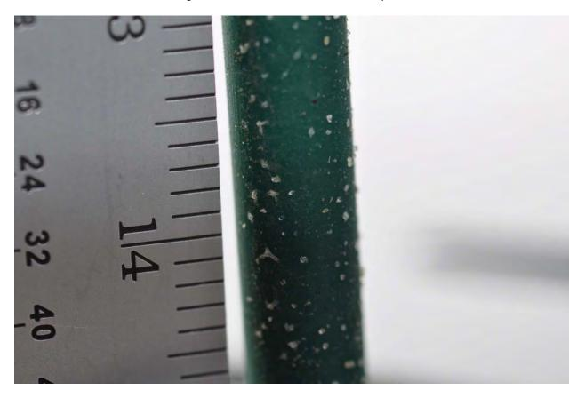
Figure B55. Fuse Bonded PVC Coated Galvanized Wire Coupon
