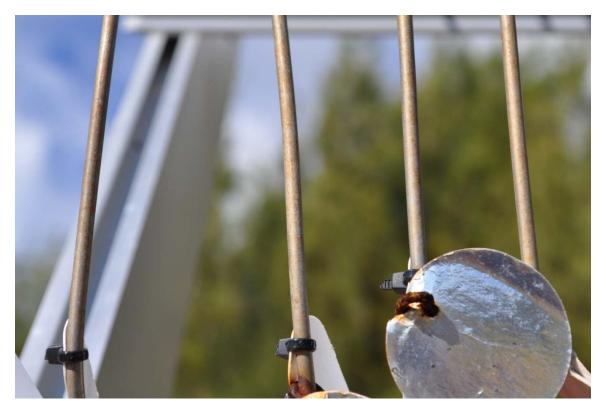
Figure B94. Stainless Steel Wire Coupon
