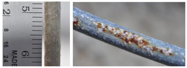
Figure 23. Standard galvanized steel wire coupon at FRF (left) and KTA (right) after 12 months of exposure.
