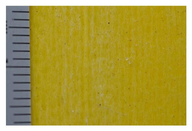
Figure B42. FRP Railing Coupon
