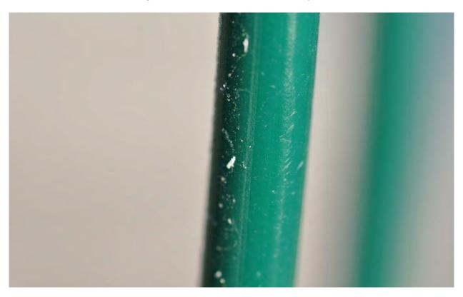
Figure B167. Fuse Bonded PVC Coated Galvanized Wire Coupon
