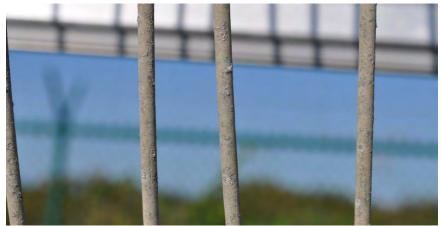
Figure B31. Standard Galvanized Wire Coupon
