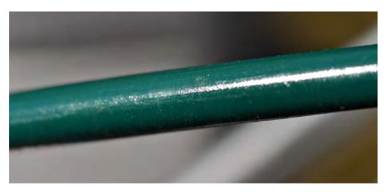
Figure B175. Standard PVC Coated Galvanized Wire Coupon
