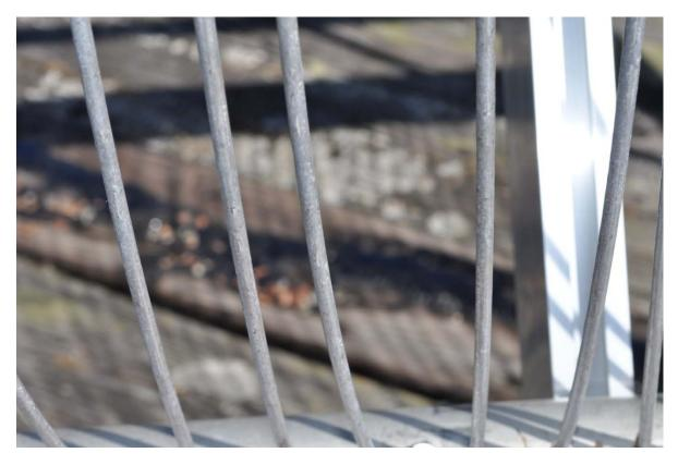
Figure B143. Aluminized Steel Wire Coupon
