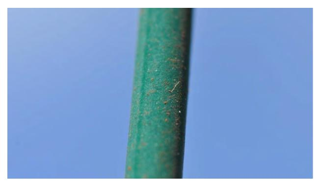
Figure B105. Standard PVC Coated Galvanized Wire Coupon
