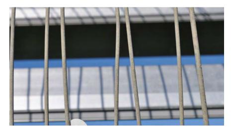
Figure B33. Aluminized Steel Wire Coupon
