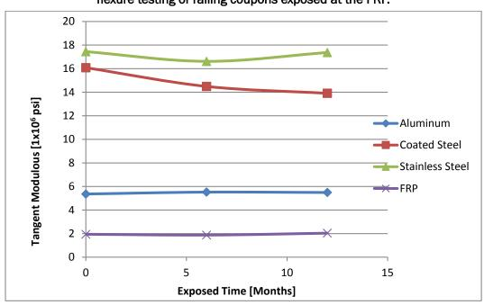
Figure 48. Tangent modulus of elasticity calculated from flexure testing of railing coupons exposed at the FRF.
