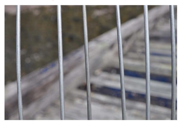
Figure B147. Stainless Steel Wire Coupon
