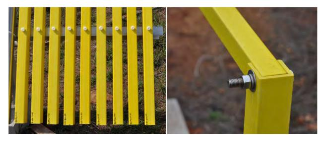
*Figure B68.* (Left) FRP railing coupons. (Right) FRP railing test section.
