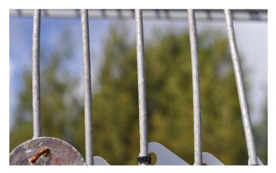
Figure B88. Aluminized Steel Wire Coupon
