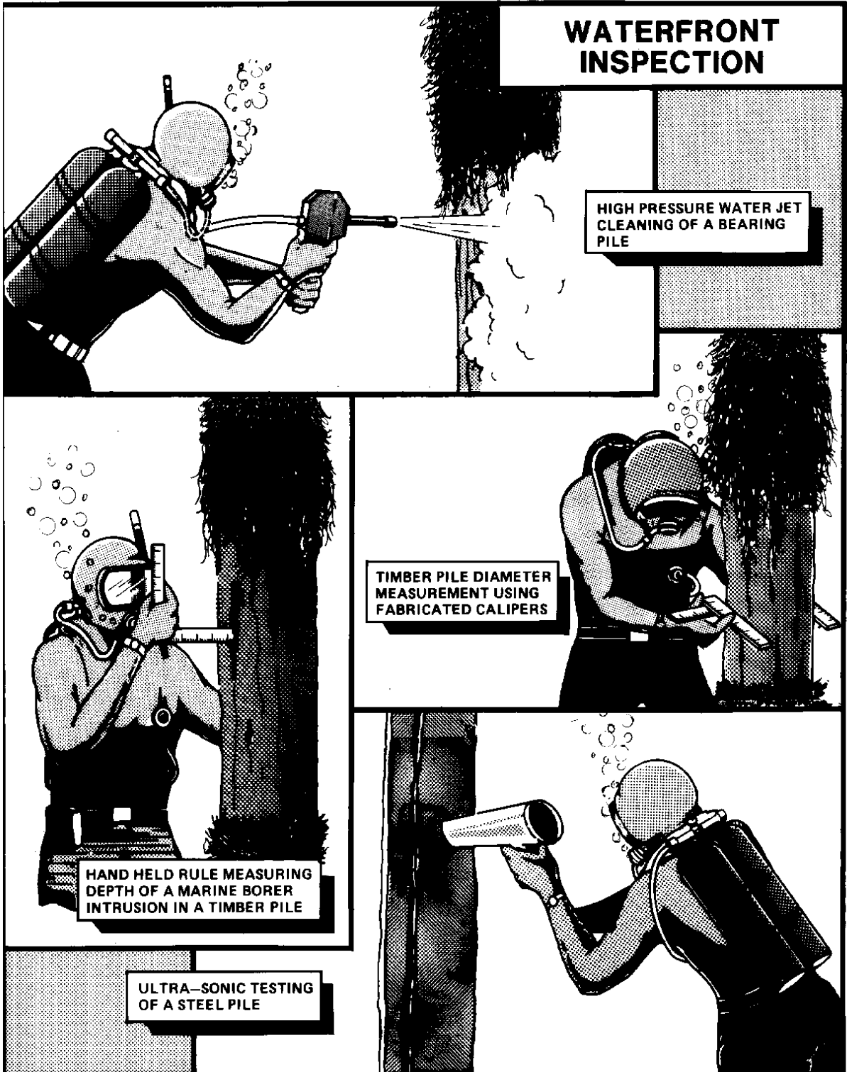
Figure 5-2 Tools and Equipment Used for Waterfront Inspection
