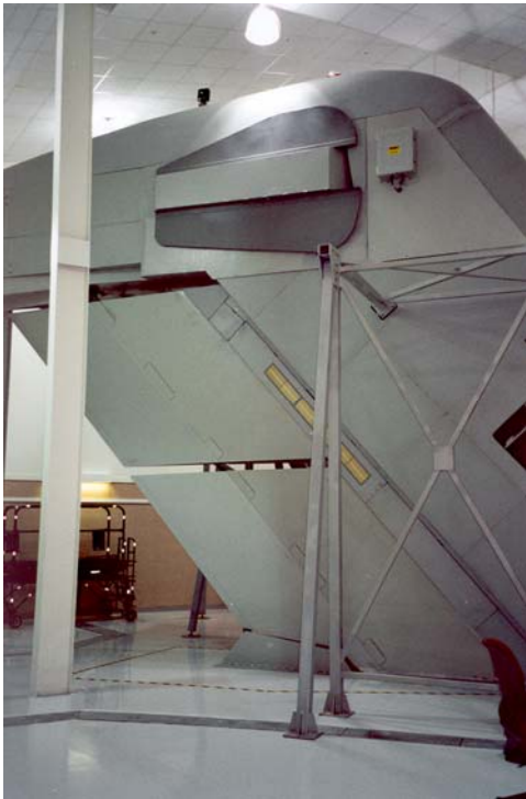
Figure 3.16: Vertical Stabilizer Training Device
