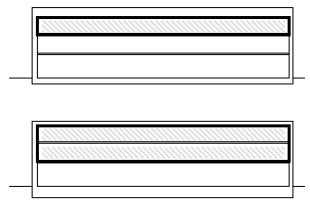
**Scenario 1:** Only the third floor is undergoing construction (shaded), so it can be considered a complete interior space by itself, and the LEED project boundary will be limited to that floor.
