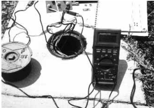
Figure 1.7. Measuring Output Current of Galvanic Anode.
