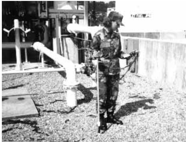
Figure 1.1. Using Data Logger for Close Interval Survey.
