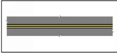
Figure C-4. Dashed Taxiway Edge Line Marking
