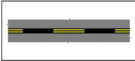
Figure C-4. Dashed Taxiway Edge Line Marking
