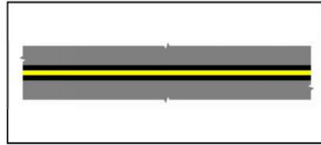
Figure C-6. Taxiway Centerline Marking
