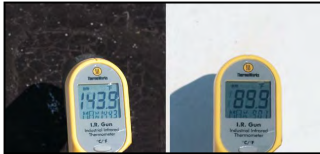
Figure 1: Dark vs. Cool Roof Surface Temperatures
