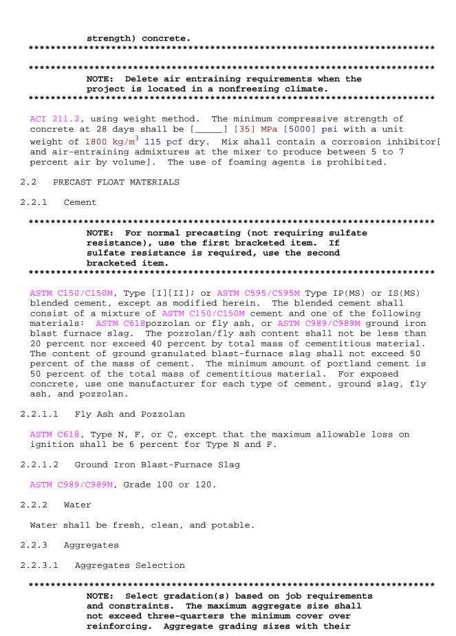
general grading ranges are as follows: Size 57 ( 25 mm one inch to No. 4 sieve), Size 67 ( 20 mm 3/4 inch to No. 4 sieve), and Size 7 ( 12 mm 1/2 inch to No. 4 sieve).
