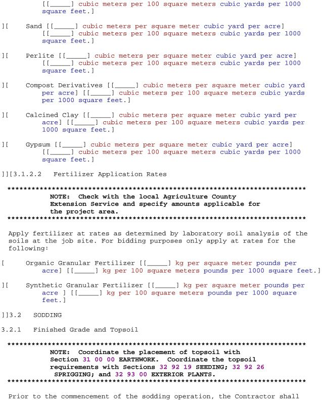
Prior to the commencement of the sodding operation, the Contractor shall verify that finished grades are as indicated on drawings; the placing of topsoil, smooth grading, and compaction requirements have been completed in accordance with Section 31 00 00 EARTHWORK.
