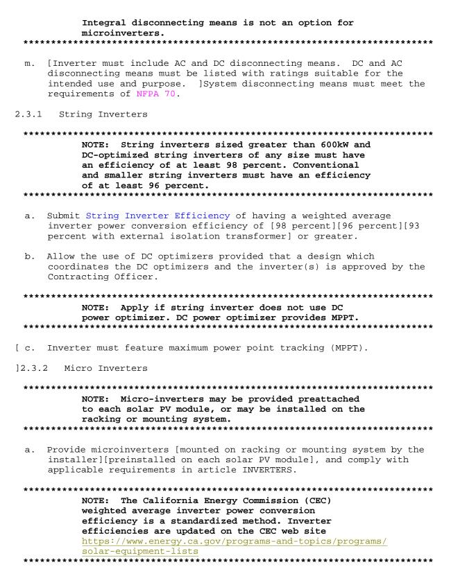
b. Submit Microinverter CEC Efficiency as verified by CEC SAND2007-5036 of having a weighted average inverter power conversion efficiency of 96 percent or greater.
