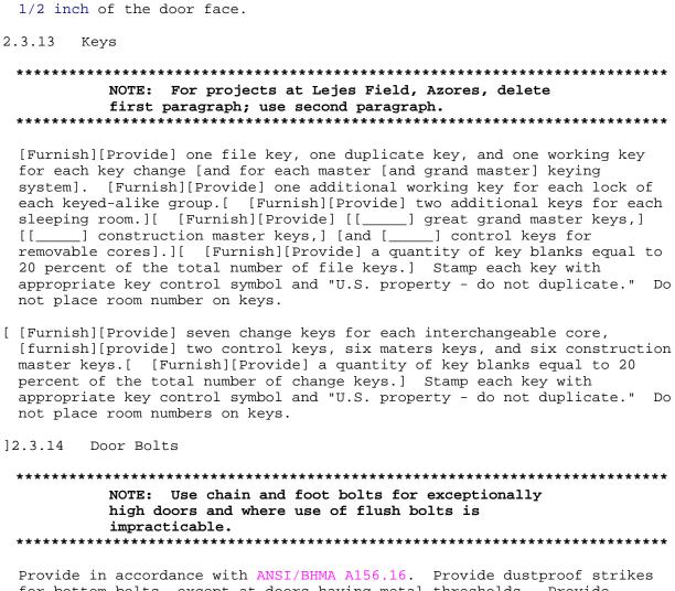
Provide in accordance with ANSI/BHMA A156.16. Provide dustproof strikes for bottom bolts, except at doors having metal thresholds. Provide automatic latching flush bolts in accordance with ANSI/BHMA A156.3, Type 25.
