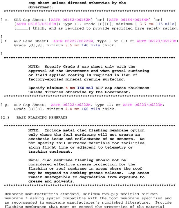
membrane flashing system compatible with the roof membrane specified and as recommended in membrane manufacturer's published literature. Provide flashing membranes that meet or exceed the properties of the material standards specified for the modified bitumen [base][, interply] and cap sheet, except that flashing membrane thickness must be as recommended by the membrane manufacturer.[ Provide metal clad flashing membrane that complies with ASTM D6298].
