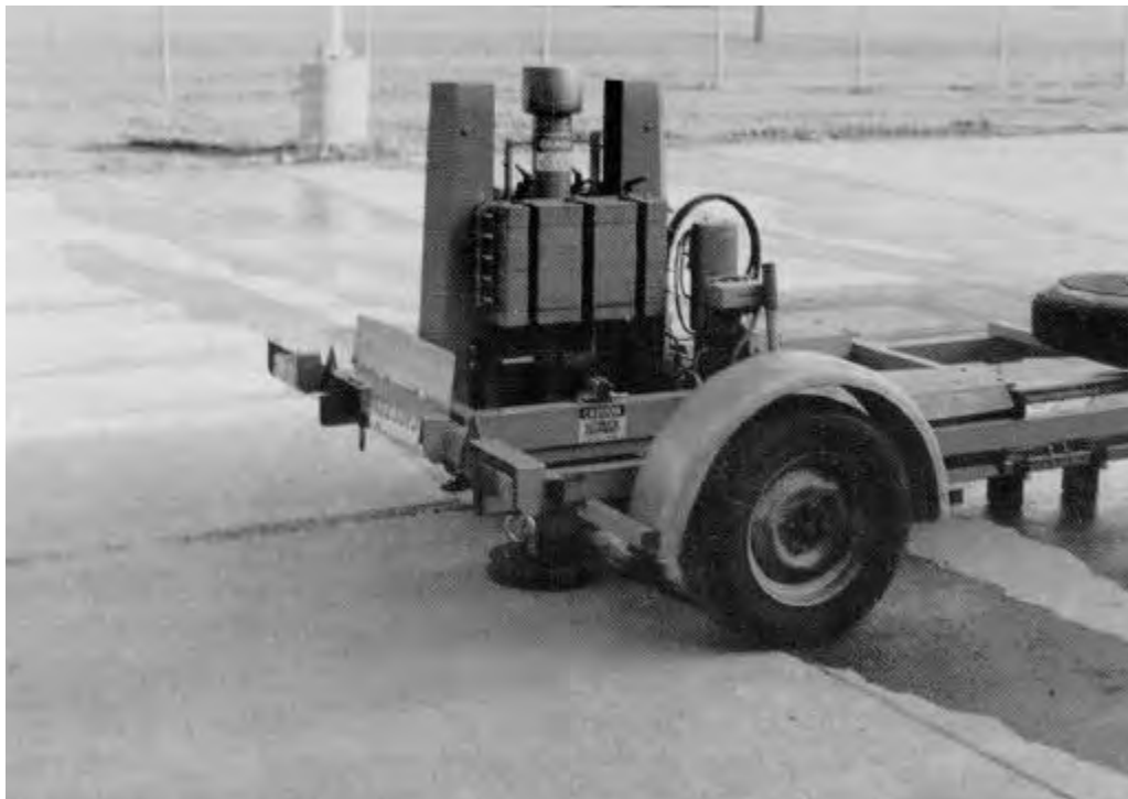
Figure 7.1. Falling Weight Deflectometer
