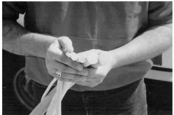
Figure 9.2. Examples of backer rod materials
