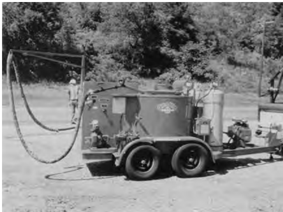
Figure 8.1. Hot-applied sealant application equipment
