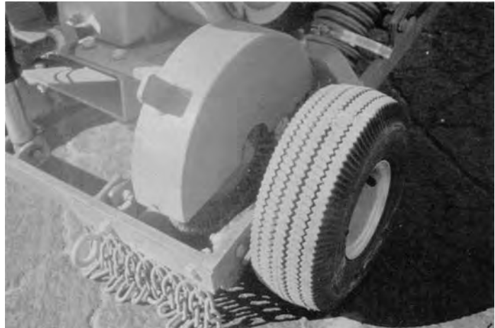
Figure 6.8. Wire brush equipment
