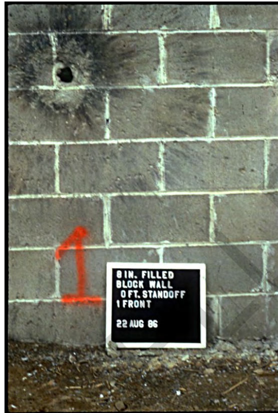
Figure 2-3. Shaped Charge Penetration of Masonry
