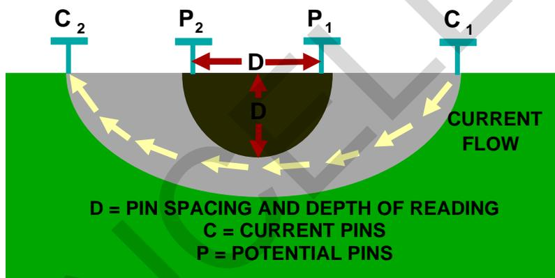
The soil resistivity is calculated from the indicated reading by using the following formula:
