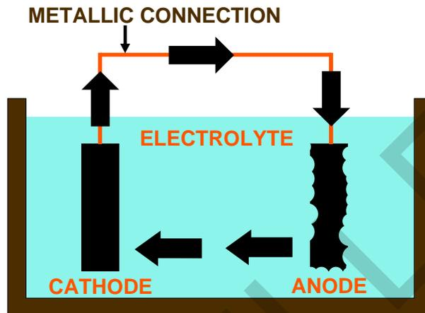
The corrosion reaction should be considered as a cyclic phenomenon where each of the components of the cell must be present and functioning in order for the overall electrochemical corrosion reaction to proceed. If any one of the components of the electrochemical cell are removed or if the individual reactions at either the anode or the cathode can be prevented from occurring then the entire corrosion process can be prevented.
