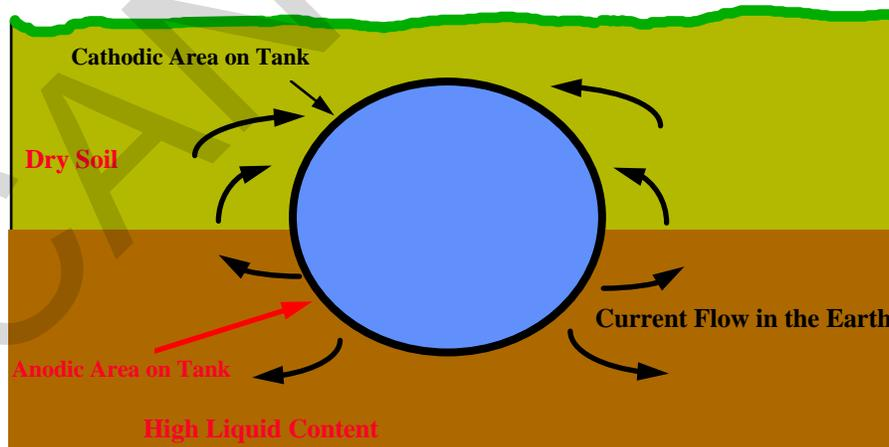
2-2.2.4 **Non-Homogeneous Soil.** Pipelines or tanks that are exposed to an electrolyte that is not homogeneous exhibit different electrical potentials in the different
