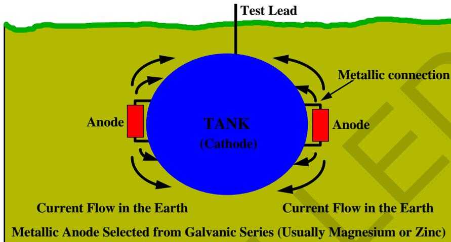
For the protection of underground structures such as pipelines, the anodes are not usually attached directly to the structure, but are placed in the soil, evenly distributed a short distance from the pipeline, and are connected to the pipeline by a wire, usually through a test station. This type of sacrificial anode system is shown in Figure 2-19.
