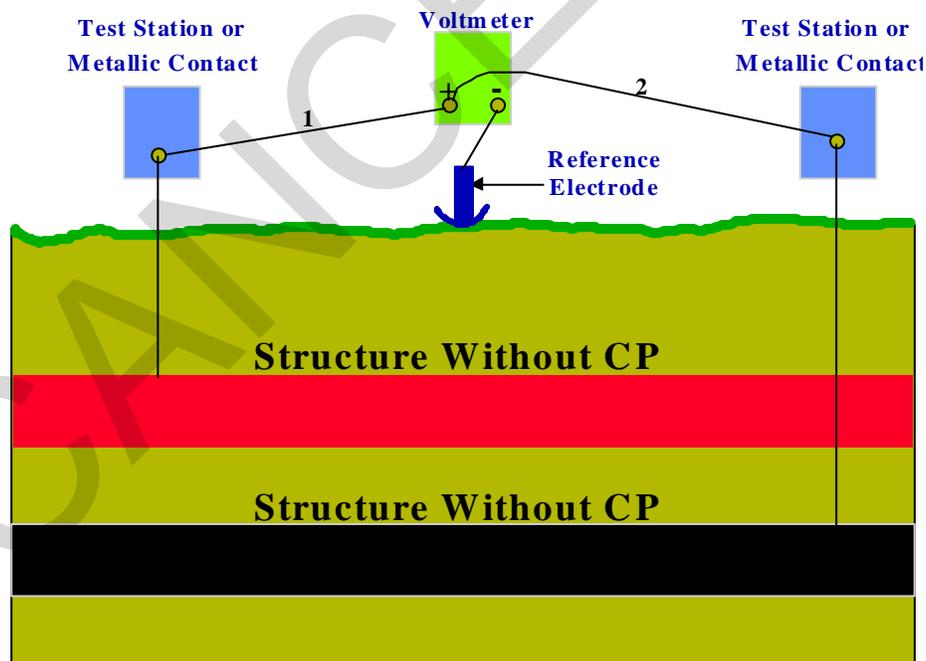
7-9.3.1 If the two potential measurements are significantly different (over 25 mV), the two structures are not metallically shorted together. Under normal conditions, steel structures should have a potential between approximately -0.35 volts DC and -0.65 volts
