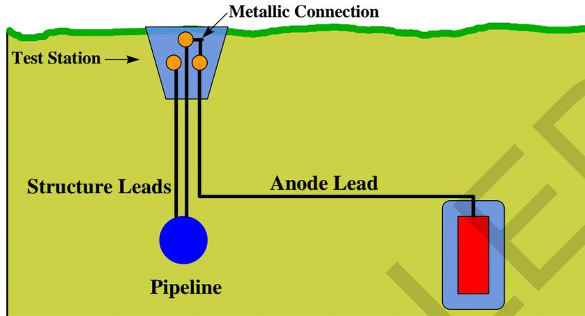
Test stations are used to conduct many different tests in cathodic protection systems. For galvanic anode systems, the most common test station measures the potential of the structure nearest the anode, the potential of the structure farthest from the anode, the potential of the anode, and the amount of current being supplied by an anode or group of anodes. The connections in this type of test station are shown in Figure 2-23.
