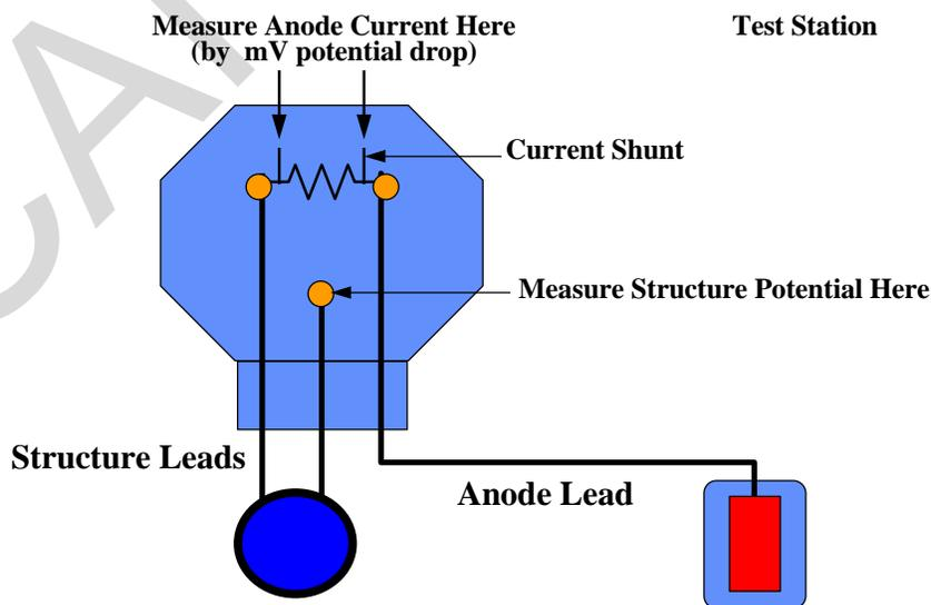
Normally, a test station has three wires as shown in Figure 2-23. Some test stations may not have current shunts, may not have a separate structure potential measurement lead, may have multiple anode leads, may just have one structure lead (anodes connected directly to structure), or there may be multiple anodes with a single lead.
