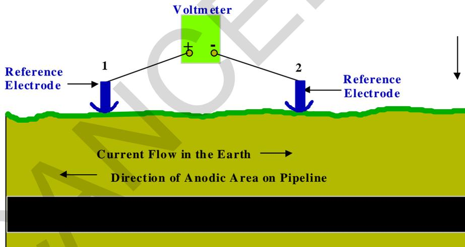
Figure 7-11. Negative Reading for Cell-To-Cell Survey
