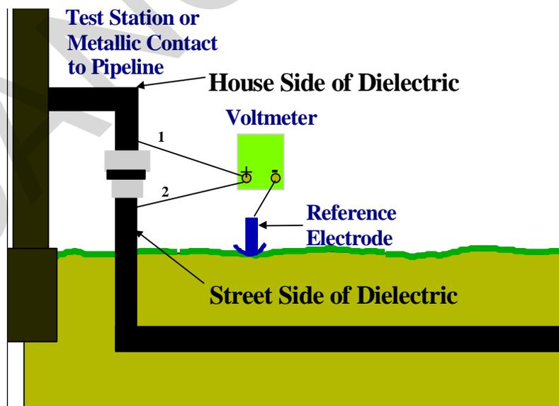
7-7.1.1 If the two potential measurements are significantly different (over 10 mV), the
