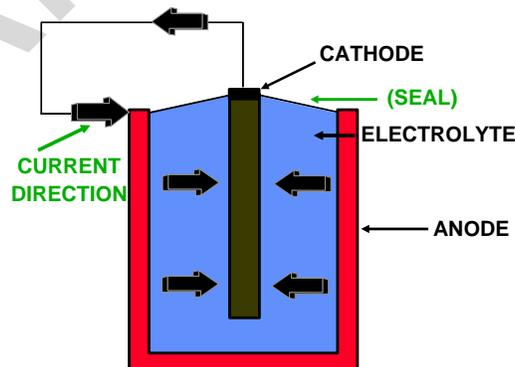
2-1.1.6 **Anode Reaction.** At the anode the metal atoms give up one or more electrons and become metal ions. In chemical shorthand the general formula for this reaction is written:
