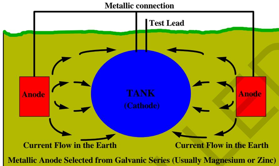
2-6.1 **Galvanic Anode Types.** There are three materials that are commonly used as galvanic anodes: magnesium, aluminum alloy, and zinc. Each material has different grades or types available. Each type is available in a multitude of sizes and shapes. For specific information on design, and information on types, sizes and shapes, consult MIL-HDBK-1004/10.
