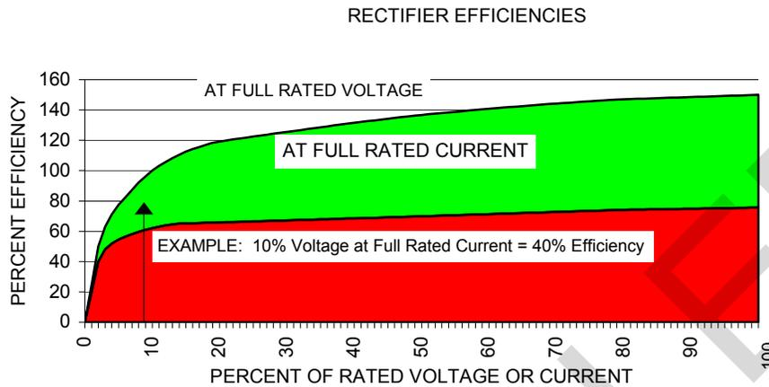
7-6.3 **Expected Efficiency.** The expected efficiency of a rectifier depends on the type of AC power (single or three-phase), Type of rectifying elements (selenium or silicon), type of rectifier (bridge or center tap), and the percent of load of the unit. The selenium bridge rectifier is the most common unit. The selenium inherently is less efficient due to the voltage drop of the rectifier elements (and resultant heat). Selenium ages with time and becomes less efficient as time passes.
