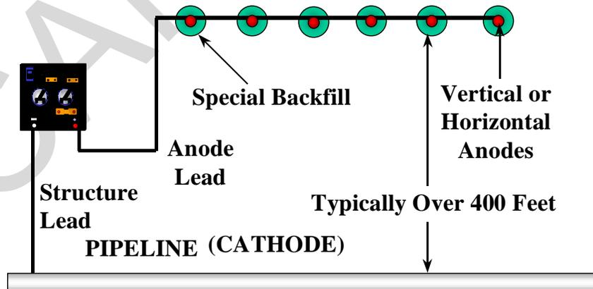
**2-7.3.2 Horizontal Remote Impressed Current CP Systems.** These systems are commonly used for pipelines in remote areas where a rock stratum is located near the surface or where other soil conditions would require horizontal installation to ensure the
