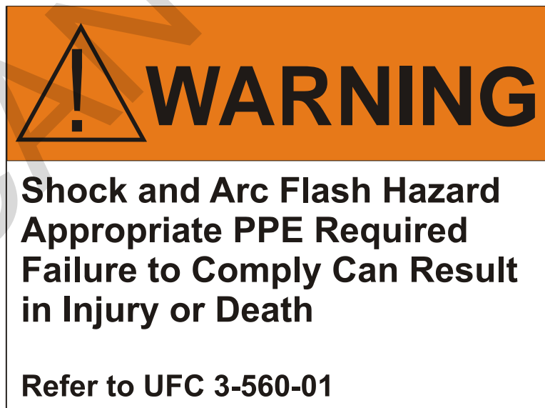
Figure 1-3 Typical Arc Flash Warning Label
