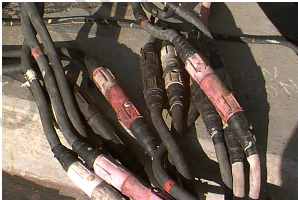
Figure 13-11. 480 Volt Shore-Cable to Ship-Cable with Single-Pole Connection
