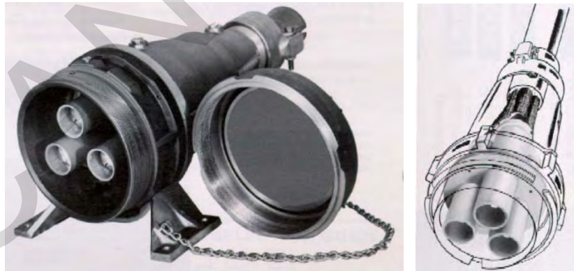
Figure 13-19. High-Voltage Shore Receptacle
