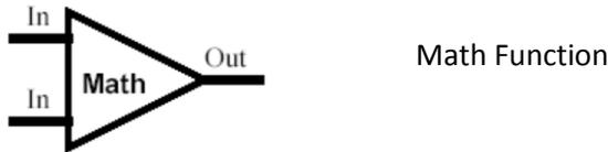
This logic block represents a variety of mathematical functions. It takes two or more analog inputs and produces an analog output. Some common functions for this block are shown in the table below.
