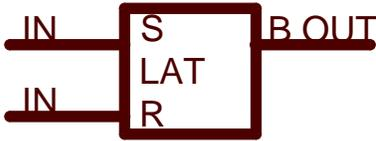
This function block represents a latch. The latch has 2 binary inputs, a set input and a reset input, as well as a single binary output. Once set (by a TRUE value at the Set input), the latch's output remains TRUE until reset (by a TRUE value at the reset input). Likewise, once reset, the output remains FALSE until set by a TRUE value at the set input. Essentially, the latch remembers whether it was last Set or Reset.
