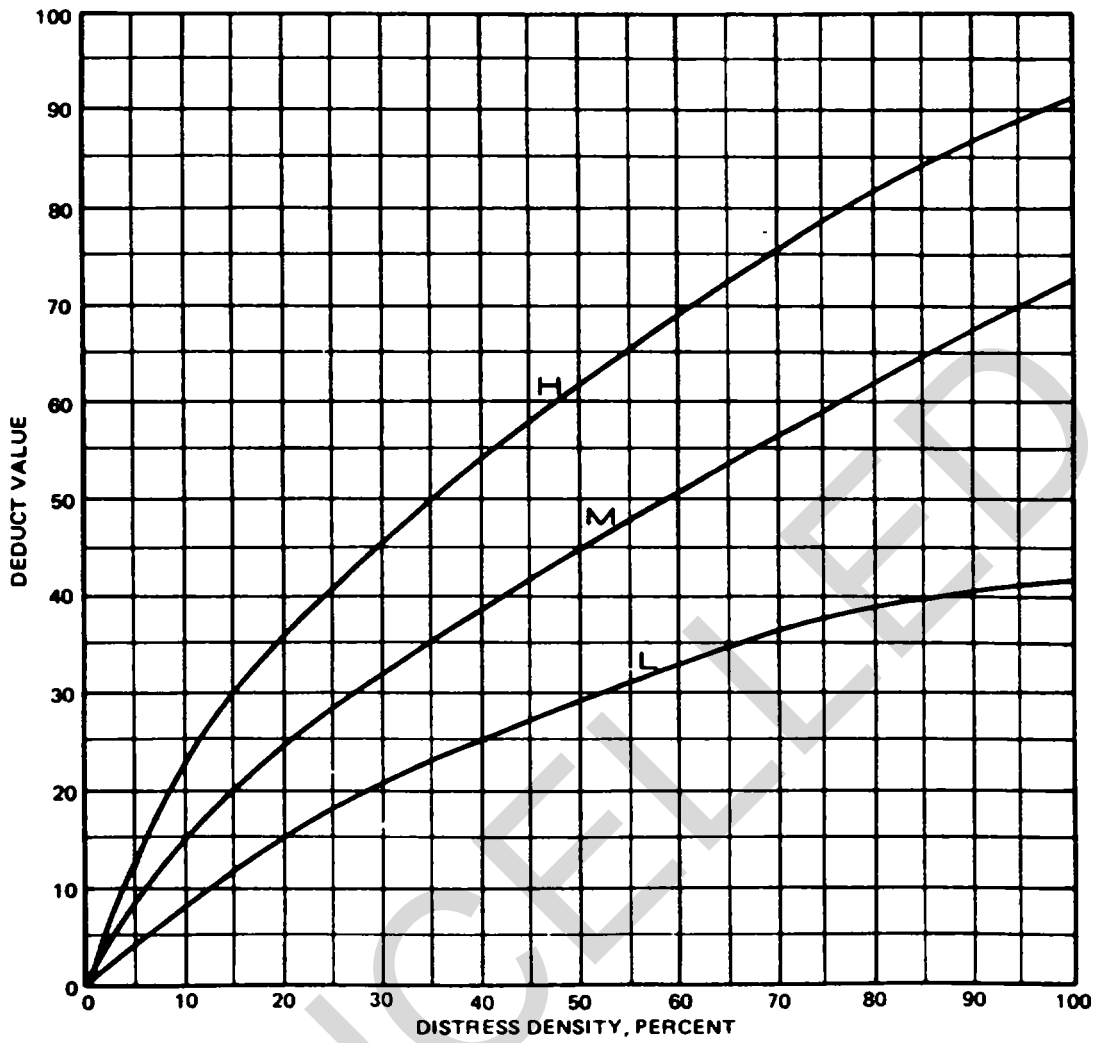
Figure 5-3. Rigid pavement deduct values, distress 62 corner break.
