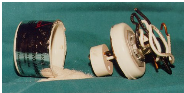
Figure 3 Unlisted Surge Protector
