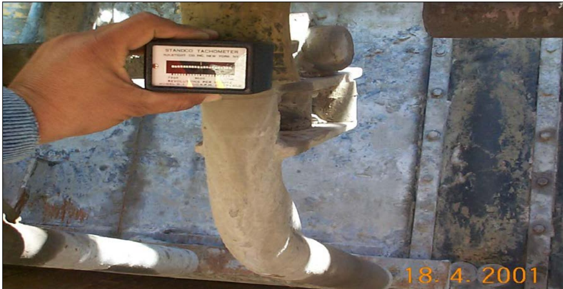
Figure 4-98 Optical Wedge Sicker for Measuring Vibrator Amplitude
