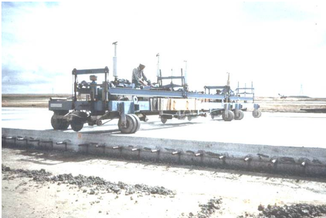
Figure 4-142 Saw Cutting Machine With Multiple Blades
