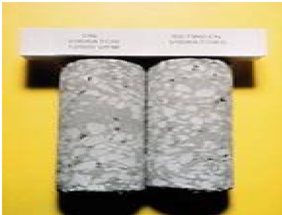
Figure 4-101 Cores Illustrating Segregation from Over Vibration (Core on Left Was Taken Along Vibrator Alignment, While the Core on the Right Was Taken Between the Vibrators. Vibration Frequency = 12,000 VPM.)
