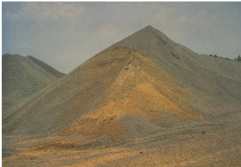
Figure 3-8 Contamination of Stockpile from Underlying Materials
