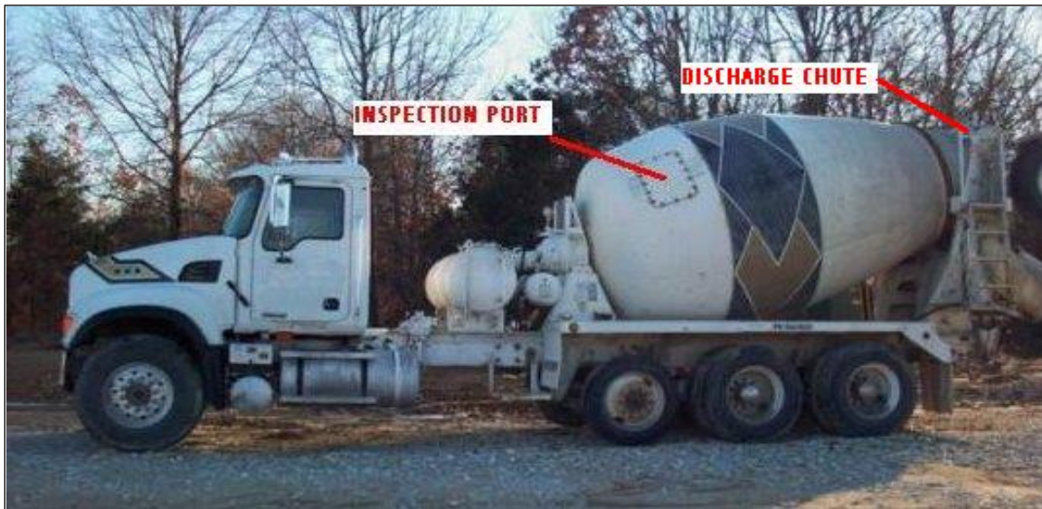
Figure 4-16 Inspection Port on Inclined-Axis Revolving Drum
