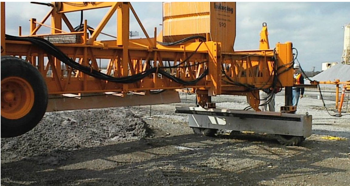
Figure 4-110 Broom Texturing Equipment
