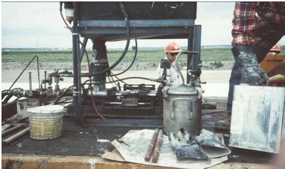
Figure 4.58 Equipment Mixing of Epoxy Grout
