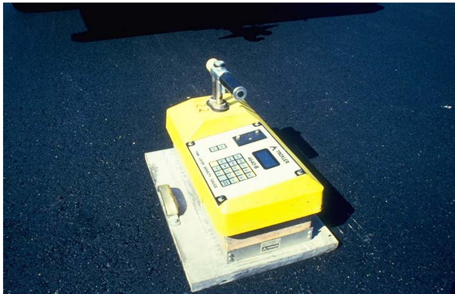
Figure 3-49 Density Measurement with Density Gage
