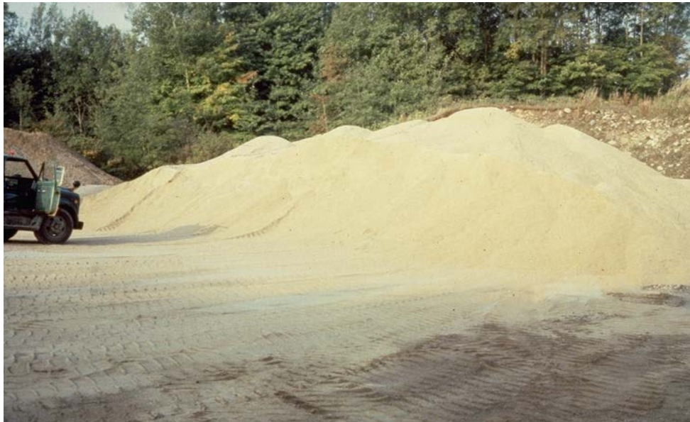
Figure 3-2 Typical Aggregate Stockpile
