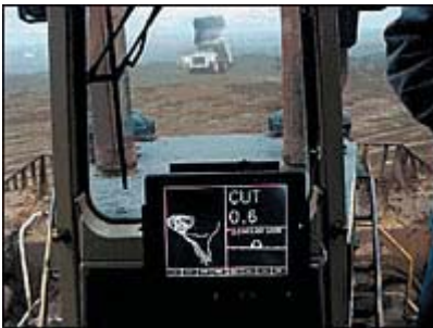
Left: A view out from a dozer using a GPS system for site work. Right: A schematic diagram showing how the GPS works on-site.
