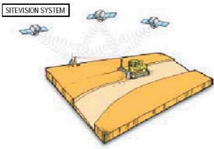
Left: A view out from a dozer using a GPS system for site work. Right: A schematic diagram showing how the GPS works on-site.
