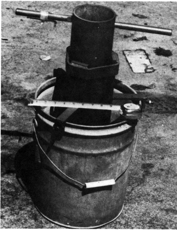
Fig. 1. Prototype tremie flow test apparatus.
