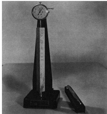
Fig. 1. Length comparator with 11-1/2-in. reference bar
