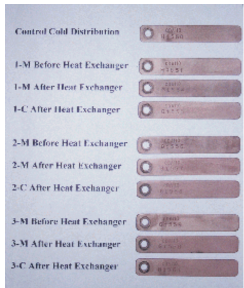
Figure C8 Corrosion Coupons after cleaning
