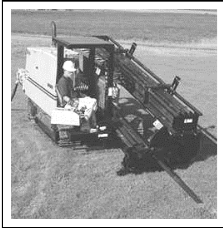
Figure 6. Directional Drill Rig On Mobile Tracked Platform.
