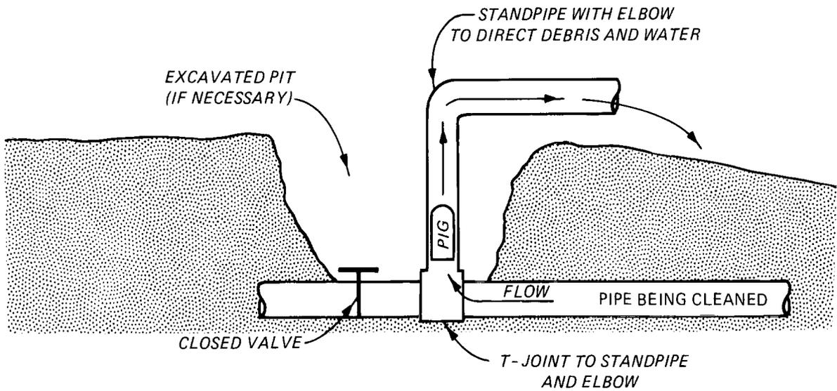
Figure 4. Typical pig retriever configuration.
