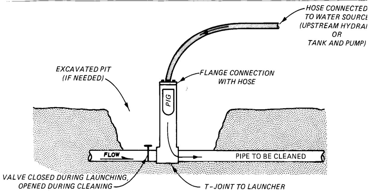
Figure 3. Typical pig launcher configuration.
