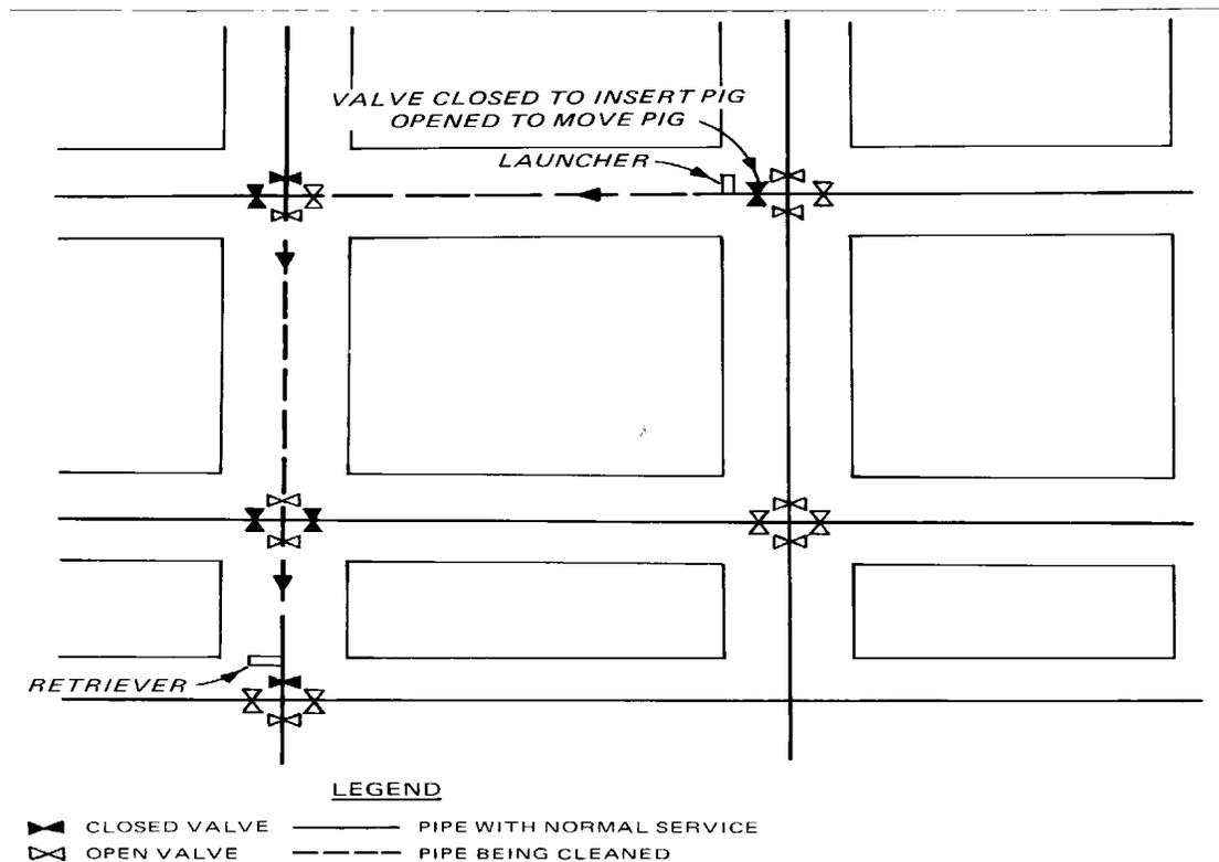
(4) A pressurized water source is necessary for inserting the pig. Pig insertion can be connecting to an upstream hydrant with a backflow preventer in line, or a small water tank 250 gal nation. The pressurized water source will force the pig from the launching joint into the water main and propel the pig through the line.
