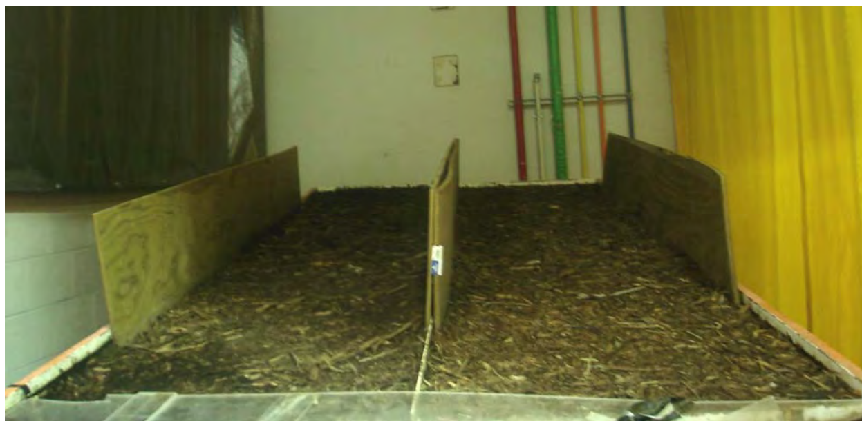
Figure B-2. Compost and mulch mix (left) and mulch cover (right) compartments with 8% slope condition, after rainfall simulator experiment.
