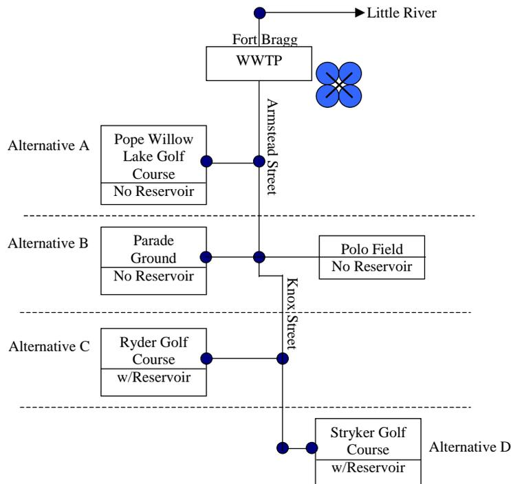
Figure A-1. Distribution schematic for Alternatives A through D.
