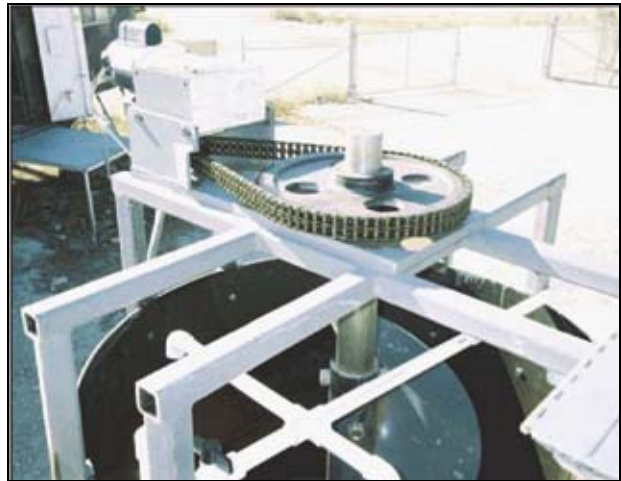
Figure A-9. Motor and sprocket.
