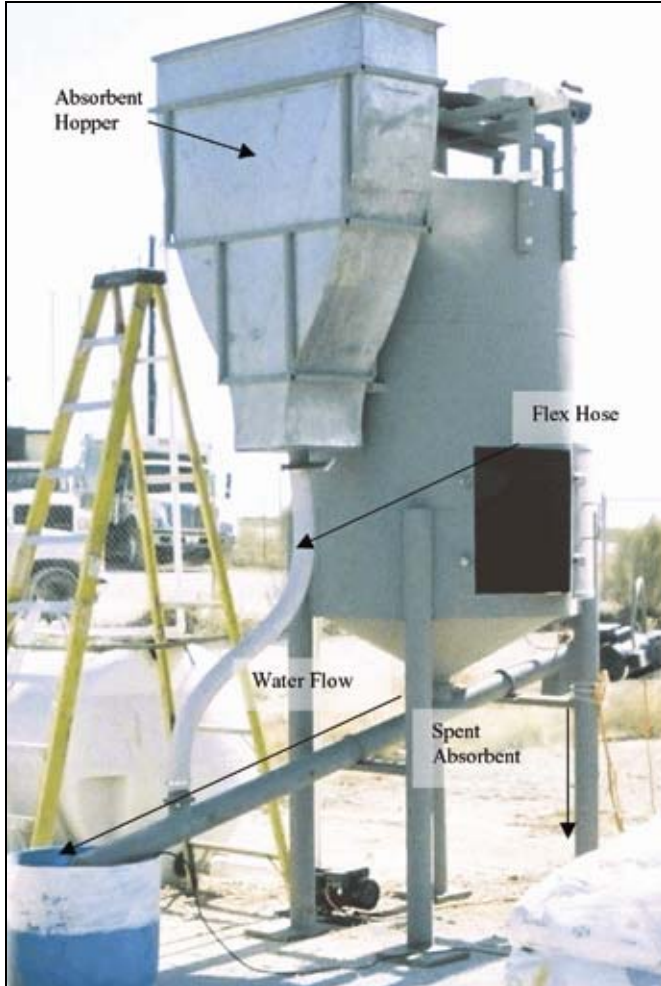
Figure A-13. Absorbent conveyor layout.
