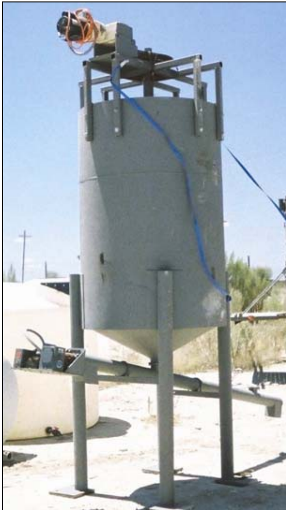
Figure A-8. Large absorbent vessel.
