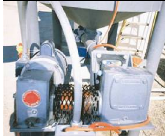
Figure A-14. Motor end of auger.
