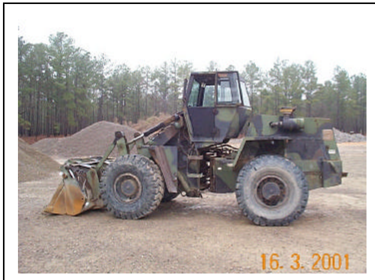
Figure 9. A Front-End Loader Is Used To Stockpile Recycled Concrete.
