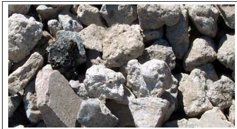
Figure 4. Crushed Concrete Aggregate.
