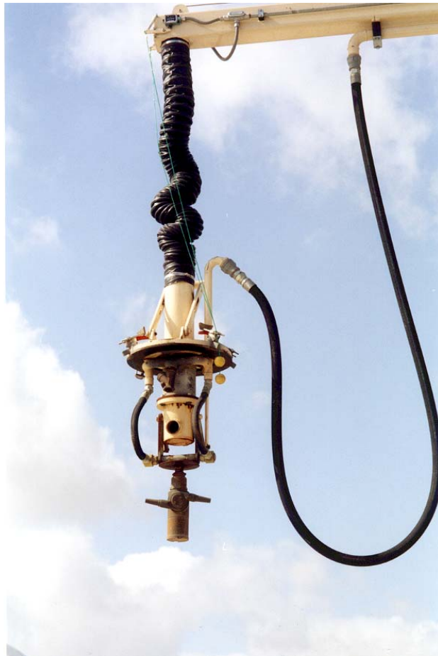
Figure 6 – Rotating spray apparatus used to clean the inside of a fuel tanker
