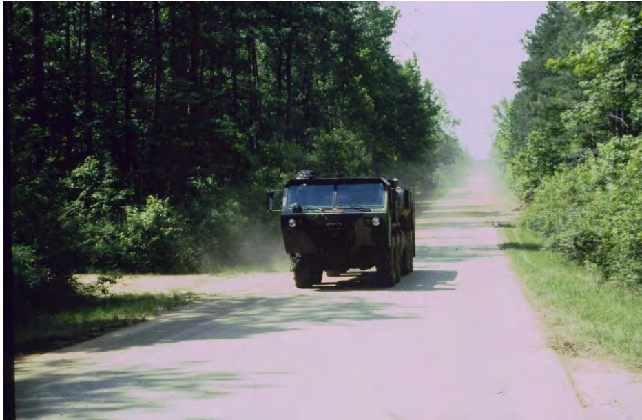
Figure C-1. Example of dust capture from Shelby truck on narrow, unpaved road that cuts through trees and vegetation.
