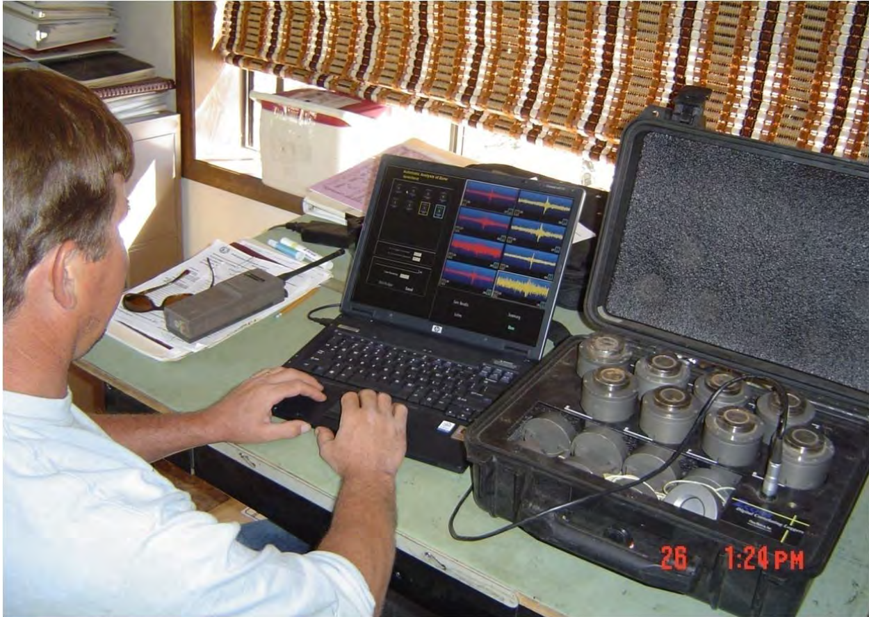
Figure A-4. A more advanced leak detection system uses software to analyze information downloaded from data loggers located on pipes within a water distribution system (Scholze 2011b).
